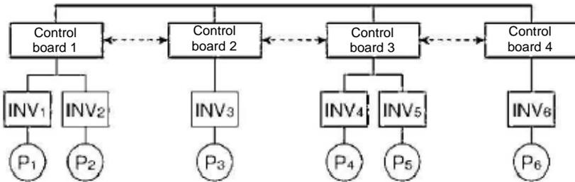
If a failure of control board 3 occurs in the drawing at left, the operation is continued by control boards 1, 2 and 4.
