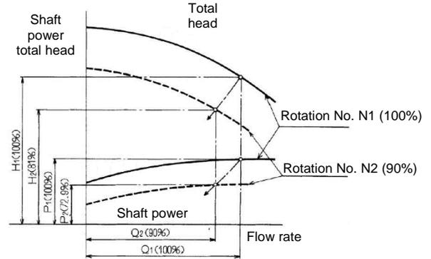
[Drawing 3-1] Relationship between the pump's characteristics and rotation speed
