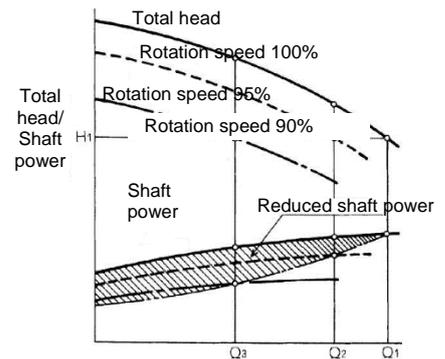
[Drawing 3-2] Comparison of shaft power at the time of rotation speed change
