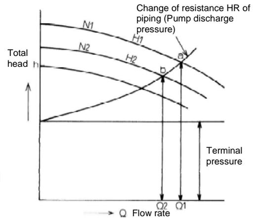
●Comparison between the total head-flow rate & shaft power-flow rate curves (Constant discharge pressure control and constant estimated terminal pressure control)
